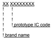
If a foreign analogue has a three-letter code before its digital (alphanumeric) number, then the corresponding two-letter code of JSC INTEGRAL is indicated before the digital number of the prototype IC with the addition of the third letter of the prototype letter code (for example, ILX) to it.
